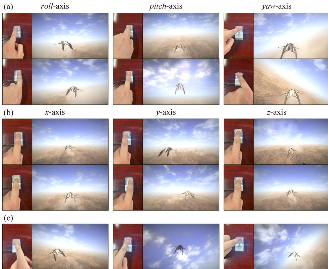
Fig. 12. Virtual aircraft flight control using OneTip. (a) Input 3-D orientation variation, and change the rotation angles of the three axes separately. (b) Input 3-D position variation, and change the translation of the three axes separately. (c) Input 6-D pose variation, and changing fingertip pose arbitrarily. Video is available [51].
